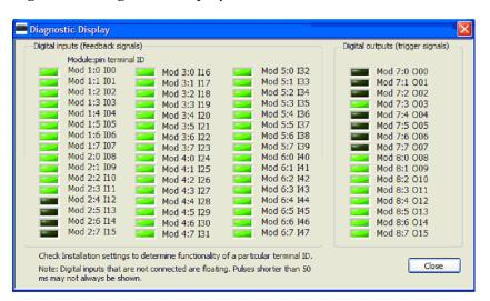
The Diagnostic Display dialogue shows the signal level of each digital input and output.
