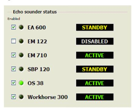
The Echo sounder status provides synchronizing status for each of the installed echo sounders
