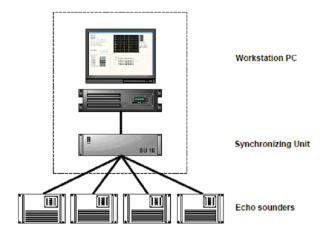
The Synchronizing Unit application provides the user interface, which allows monitoring of status, modifying settings, trigger schedule as well as performing diagnostics. The application needs to run and be connected to the Synchronizing Unit in order for the system to initialize and be operational. However, once the system is running, the application can be shut down and disconnected completely while the Synchronizing Unit continues to control the triggering of echo sounders.
