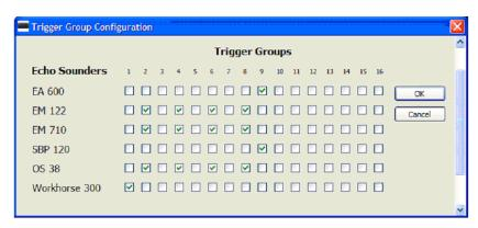
Trigger group configuration dialogue allows user to assign echo sounders to trigger groups
