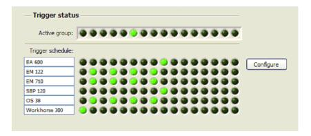
Trigger status shows which is the current group and which group each echo sounder is assigned to
