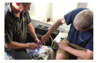
▲ HyBIS engineers Dave and Russ filling the beacons with oil so that the high pressure at the ocean floor does not cause the glass to break. Photo: B. J. Murton
