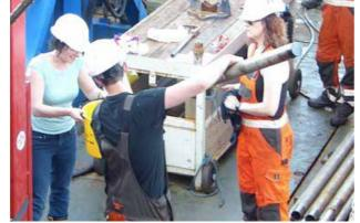
▲ Collecting fluids from the core barrels for analysis (Kate left, Joe centre and Sally right)
