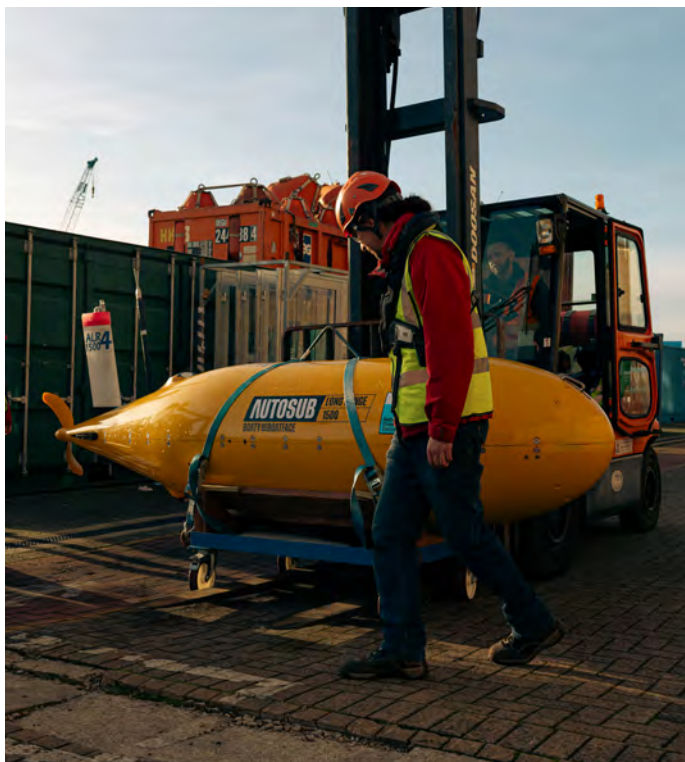
▲ Autosub Long Range (ALR), an autonomous underwater vehicle designed for deep-sea exploration and extended scientific missions.
