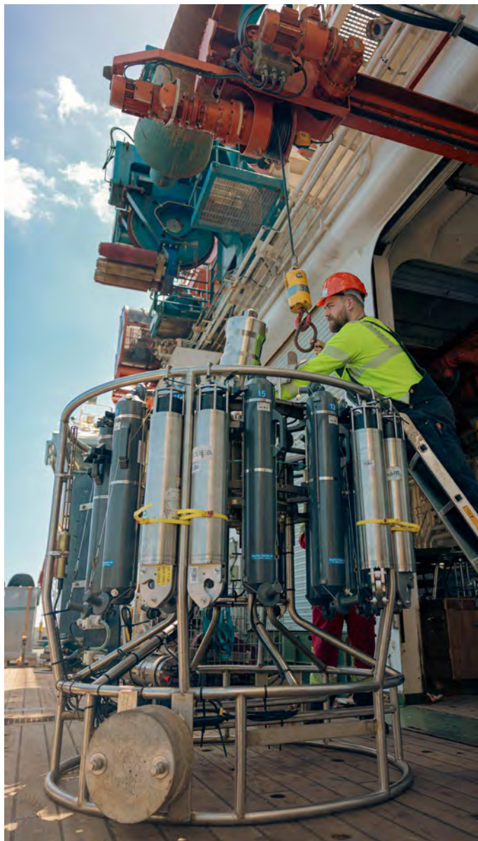
▲ Preparing a CTD instrument for deployment as part of our RAPID programme—just one of the ways we are advancing our understanding of Atlantic Ocean circulation and its role in global climate.
