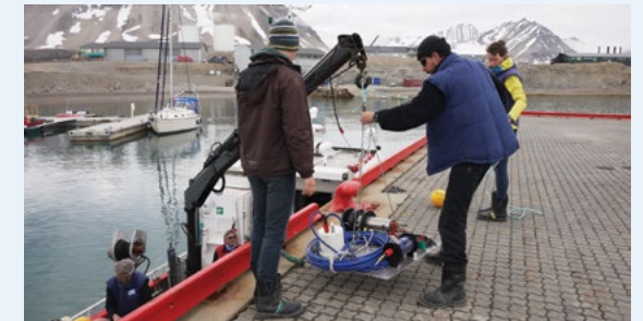
Left: The instrument was deployed at 15m depth in an Arctic fjord to establish a long-term time series of in situ measurements of algal photophysiology. Right: Autonomous acquisitions were performed every 30 minutes, with the possibility to control the system remotely through the internet to modify parameters or download data.
